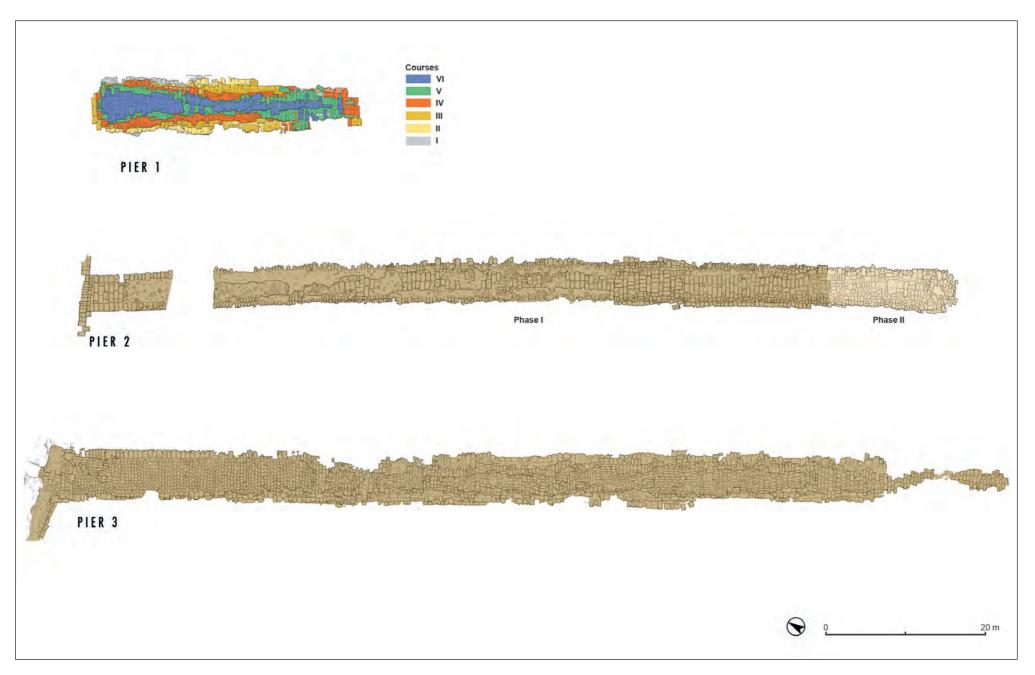
Fig. 10. Piers I, II and III, collated plans showing layers and construction phases (Plans D. Tarara; collation based on drawings by M. Kulikowska, M. Ostrowski, K. Rozmus, A. Kutiak)
