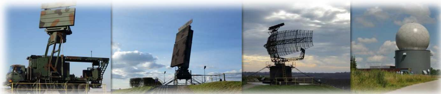
Rys. 5. Radary WRt – NUR-15M, NUR-12ME, NUR-31MK, NUR-12M
