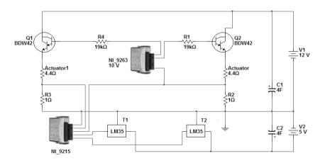
Fig. 8. Control circuit of SMA actuators Source: own elaboration.
