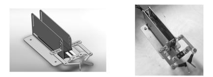
Fig. 6. 3D gripper project made in Solid Works and the real construction Source: own elaboration.
